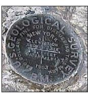
wall. The tablet is stamped "319 ALBANY 1903," recording that, at that location, Ellenville is 319.318 feet above sea level. Gary shared several sheets of information about this vertical control data that is part of a Geological Survey of the United States Department of the Interior. This Benchmark is a permanent installation, to be used as the basis for deter-
